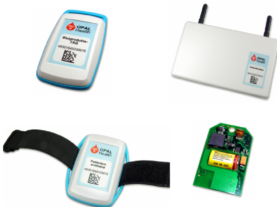
Illustration 2: Mobile tags (blood bag and patient wristband on the left) and a stationary anchor tag
